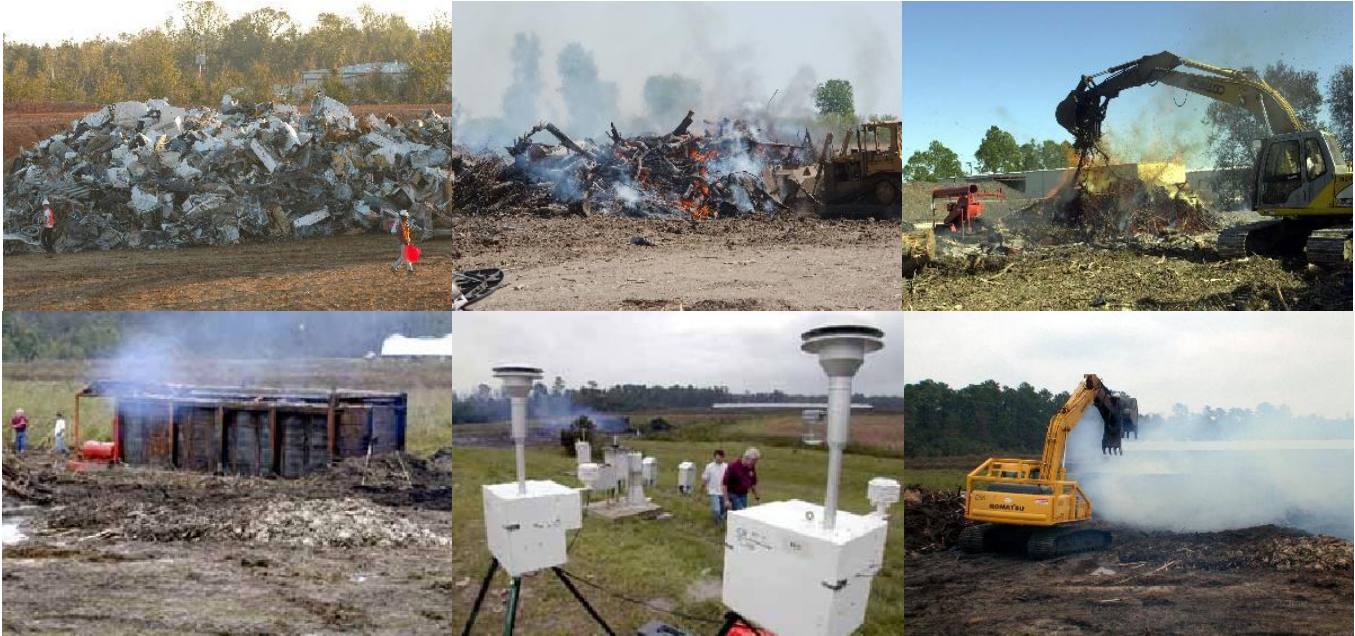
Clockwise, from upper left: Debris pile prior to volume reduction; open air, controlled burn pile; air curtain burner; portable incinerator; air monitoring equipment at burn site; open air, controlled burn pit.
